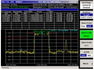
The R&S® FSL can be used for measuring both the adjacent channel power and the spectrum mask in line with the IEEE, ETSI, and WiBro standards. Using predefined limit lines, the analyzer determines, at the press of a button, whether the spectrum conforms to specified requirements. The screenshot shows the WiBro spectrum mask with pass/fail evaluation.
