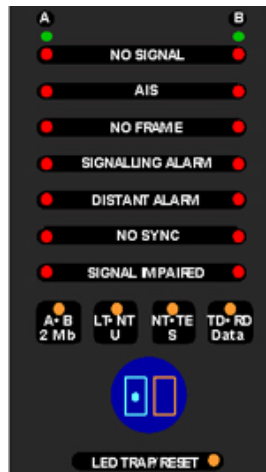
Fig 4 Line status LEDs. Detailed information on errors and alarms is shown in the display
